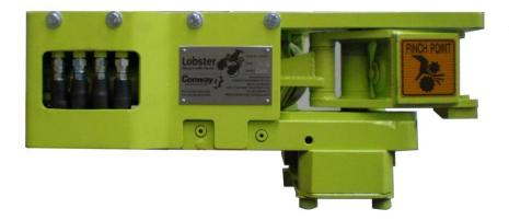
An example of a Lobster ready to be fitted to a Hydramatic Drill Rig
